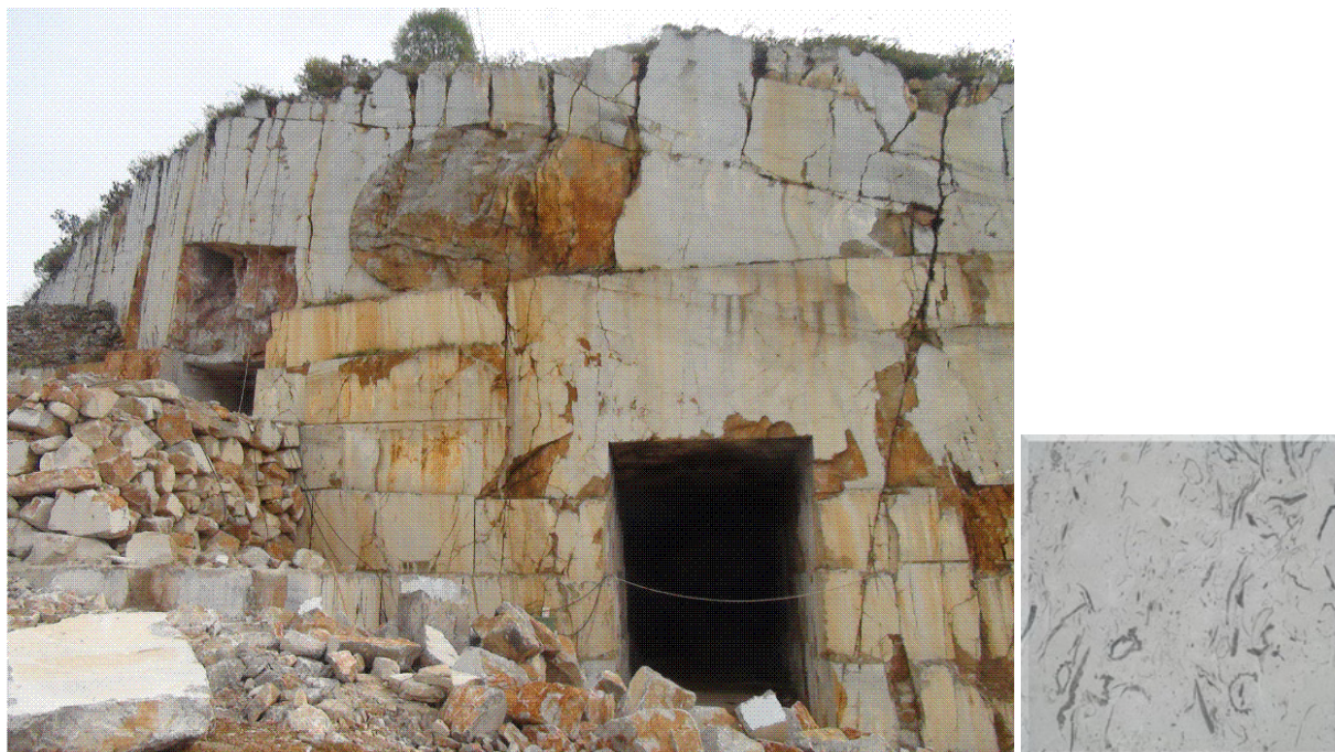
Figure 2.: High portal wall with entrance into the underground Debela Griža quarry (left), "Repen" limestone sample (right) [6].
