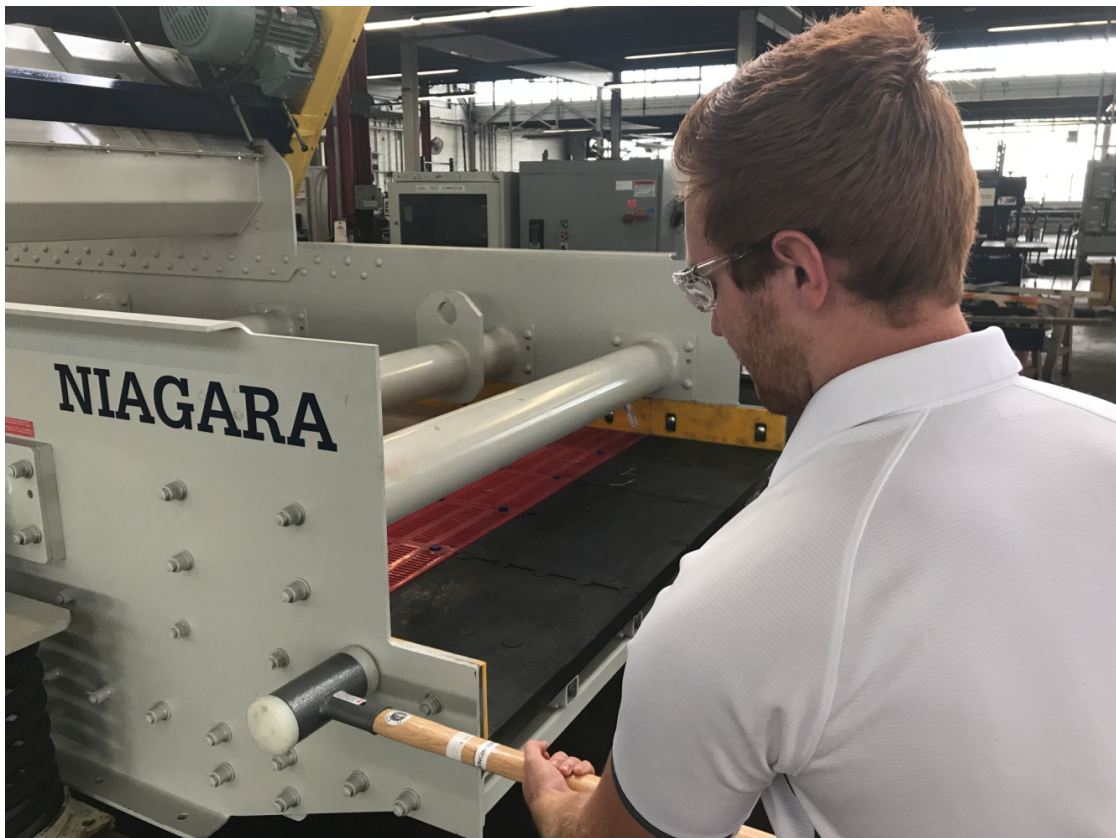
Pulse Impact Testing
